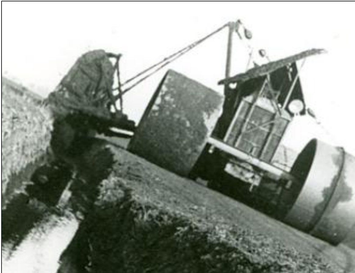
Plate 4-2: Drainage Machine Type – M.P. Field Slitter (source: https://www.bordnamonalivinghistory.ie/equipment-detail/drainage-machine/ )
