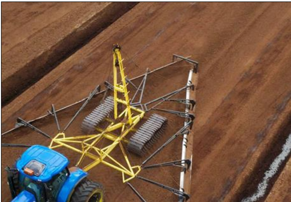
Plate 4-10: Ridging process (source: Bord na Móna)
