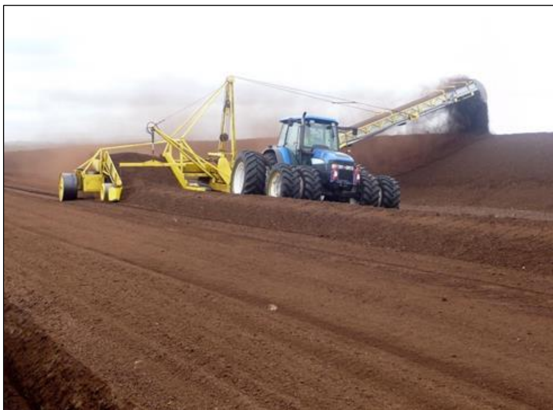
Plate 4-12: Harvesting - Peco Method (source: Bord na Móna)
